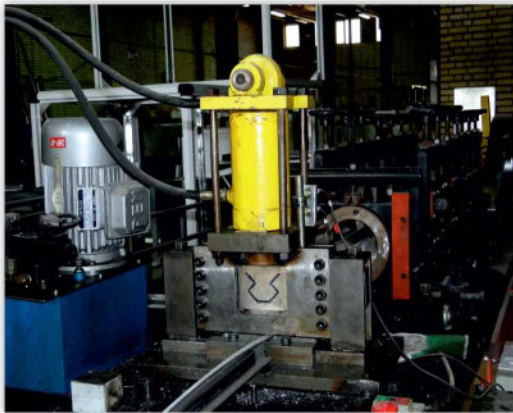
the equipment of roll forming (the frame of box)
