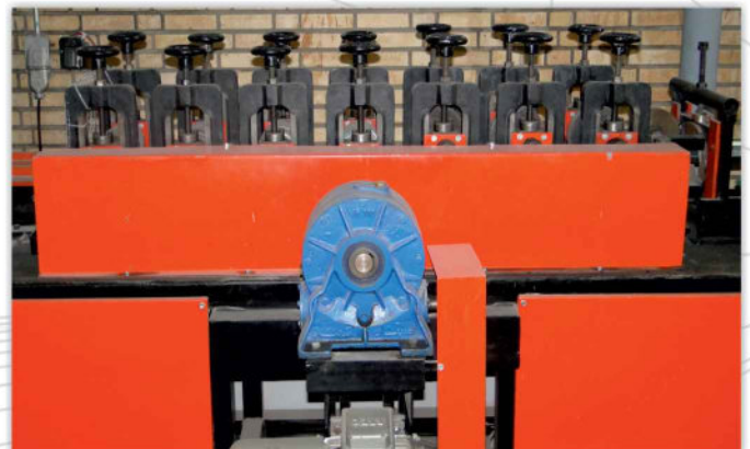
the equipment of roll forming (the frame of box)
